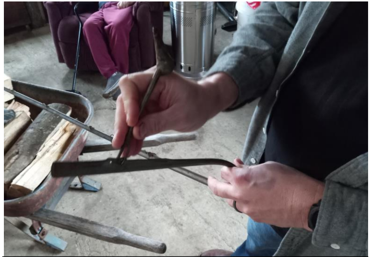
Ed displaying Brower's tin tubing system. In his right hand is the tap from the tree. That flows down into the gooseneck, which flares downward into the main tube line in his left hand.
